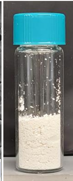
Nanoformed monoclonal antibody in dry powder
